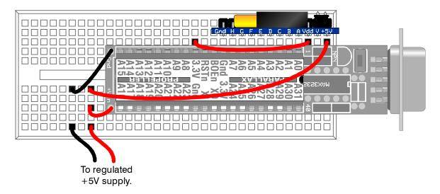
In this example, Vin is not connected. If the daughterboard requires it, an unregulated 6-9V supply could be connected to V''.
